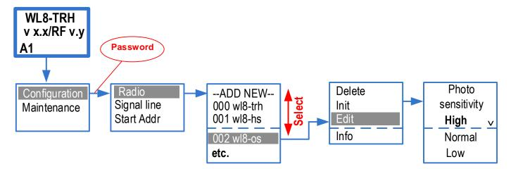
There are three sensitivity levels (High, Normal, Low) in depend on transparent air inside of room (e.g. dust, vapor). It may help to reduce probability of false alarm.
